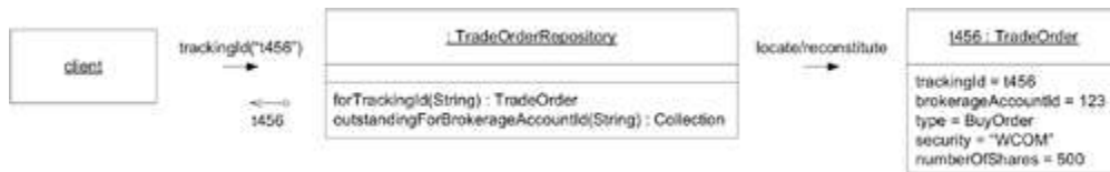
Figure 6.19. Hard-coded queries in a simple REPOSITORY
